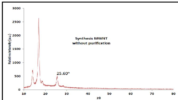
Fig. 4. XRD patterns of as grown MWNTs by chemical vapour deposition from mixture Methanol:Butanol (1:1) at  $750^\circ$ .
