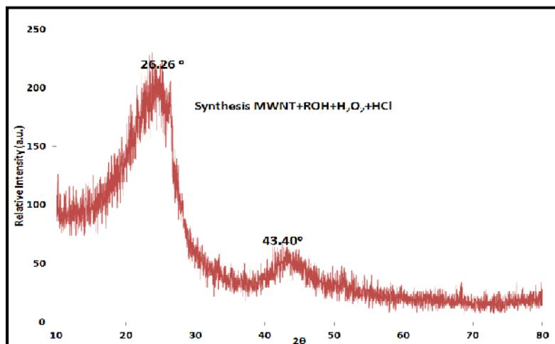
Fig. 7. XRD patterns of synthesized MWNTs after treatment with three steps ethanol, H<sub>2</sub>O<sub>2</sub> than with 5% HNO<sub>3</sub>.
