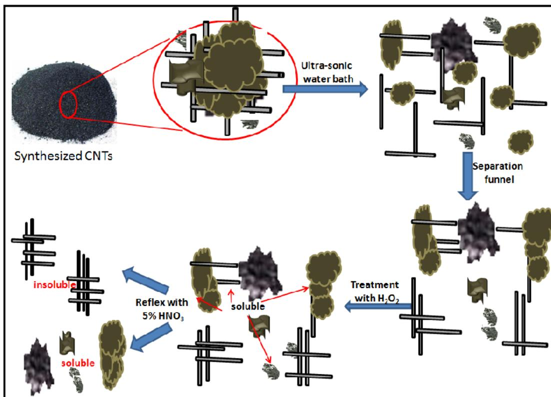
Fig. 2. Schematic diagram for the dispersion and re-distribution the sample of as grown MWNTs.
